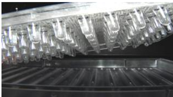
Figure 2. The inoculator showing the trough base found in products 19121, 19122, 19123, 19141, 19142, 19143, 19161, 19162, 19163, 19191, 19192, and 19193.
