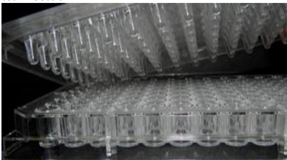
Figure 1. The inoculator showing the 96-well base found in products 19111, 19112, 19113, 19131, 19132, 19133, 19151, 19152, 19153, 19171, 19172, and 19173.
